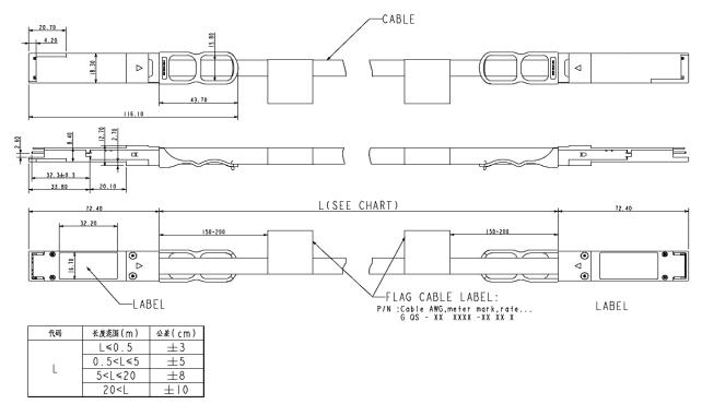
Figure2. Mechanical Specifications
