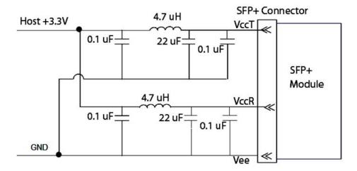
Figure 2. Host Board Power Supply Filters Circuit
